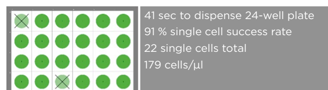
Figure 4: Single cell dispense report automatically generated from UnoControl software.
